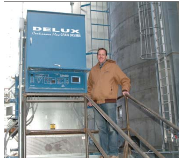
Grain Department Manager Kasey Nash is shown with the new dryer's Moisture-Link control panel.
