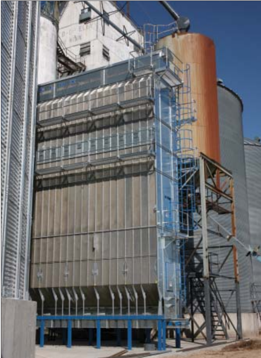
New Delux Model DPX12T grain dryer installed earlier this year at Wheaton Dumont Coop Elevator in Wheaton, MN, rated at 3,800 bph at five points of moisture removal. Photo by Danter's Photography, Alexandria, MN.
