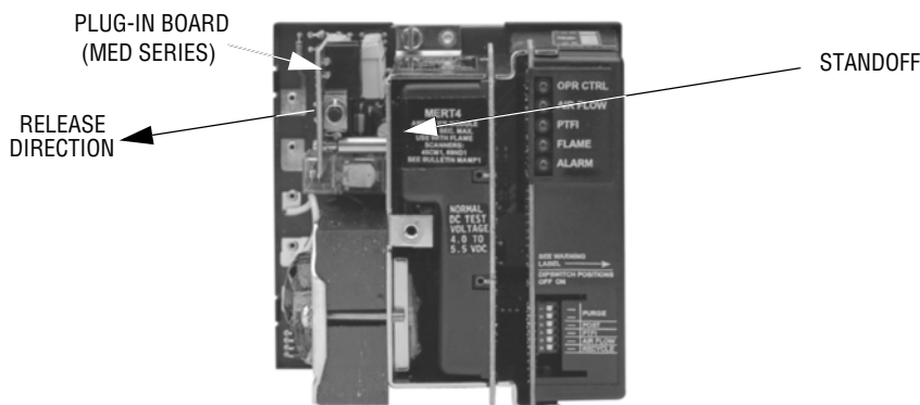
FIGURE 4. PLUG-IN BOARD LOCATION AND INSTALLATION
